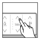
During feminine wash, press " $\land$ " in "nozzle position settings" to move the nozzle forward; press " $\checkmark$ " to move the nozzle backward.
