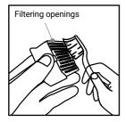
C. Use a toothbrush or other small brush to clean the odor absorber in order to remove dust.
