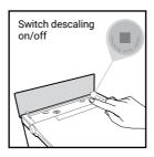
**B.** Press the descaling cycle switch to start emptying the tank. This will be accompanied by an intermittent beep. The process of emptying the tank will be completed after about 30 seconds.
